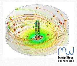
Modelling systems can be used to ensure designs are optimized such as for flow rates and particle tracking.
