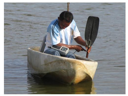
Some modern dissolved oxygen meters have an option for measuring percentage oxygen saturation. Picture by Darryl Jory.
