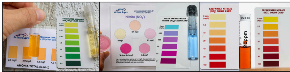
Fig. 2: Examples of colorimetric test kits for ammonia, nitrite and nitrate.
