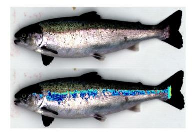
A fish with minor hemorrhaging along the body, which is not visible in a color image (upper fish), but detected with hyperspectral cameras trained to look for blood (bottom fish). Photo courtesy of Nofima.
