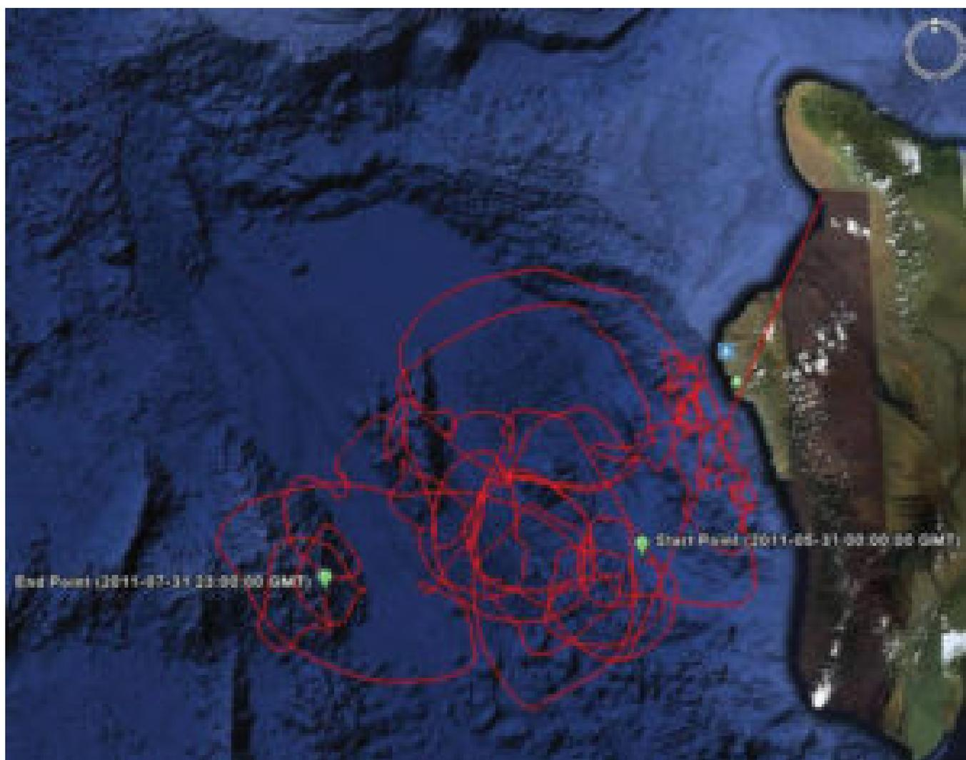
The drift track of the Veleva array shows how it moved with the equatorial eddies from May to July 2011.
