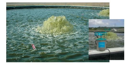
Vertical pump aerators provide good localized oxygen transfer.
