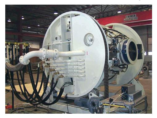
This rotating vacuum coater is moving to the discharge position. Photo courtesy of Forberg.
