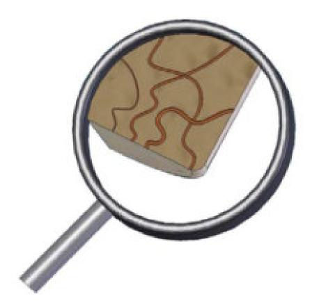
Fig. 2: As pressure is normalized, feed cells fill with oil. Illustration courtesy of Forberg.`
