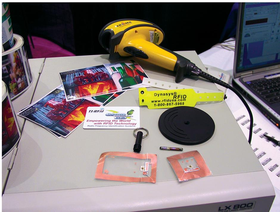
Versatile RFID tags are available with a variety of attachment configurations.
