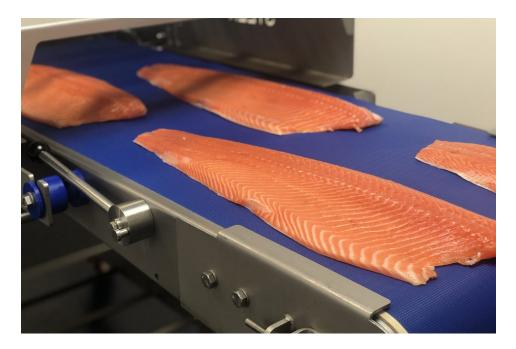
Automatic skinners can cope with a high-output capacity, are usually easy to operate and don't need much maintenance when used correctly.
