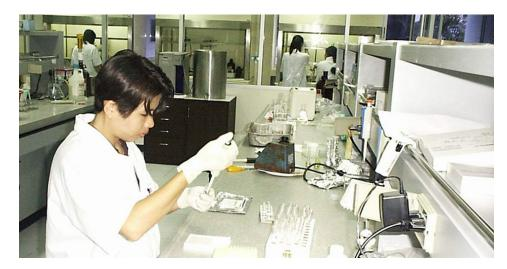
The ELISA technique is used to determine chloramphenicol residue in shrimp products.
