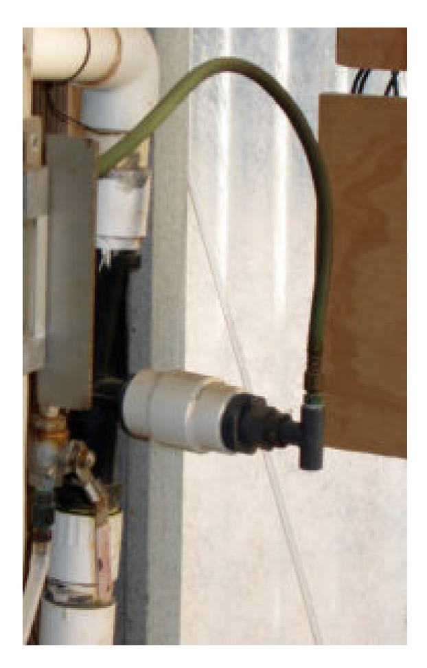
Pump-driven Venturi injectors provide limited mixing and aeration in large raceways.
