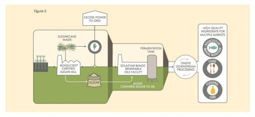
At TerraVia's facility in Brazil, microalgae converts sugars into oils and other ingredients. As a large-scale industrial process, this technology allows feed producers to predict and forecast availability, pricing, supply and other variables, with final products that don't get contaminated like a natural algae in the outdoors would.
