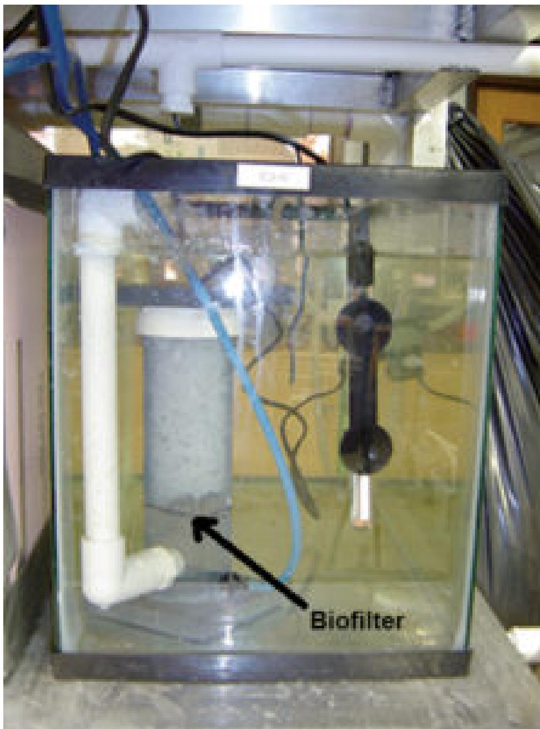
The biofilters were designed to fit into the 40-l tanks as self-contained systems.
