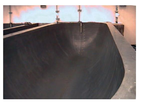
Parabolic tank designs help keep artificial feed suspended in the water column.
