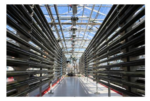
Pilot-scale photobioreactors (1,300 liters of culture). The results from this study of selenium production in the microalgae *Nannochloropsis oceanica* are currently being prepared for publication and should be available this year in the form of an open-access article. Photo by Bárbara O. Guimarães.
