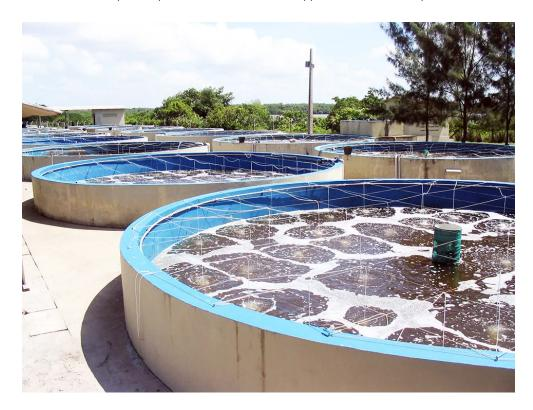
Diffused-air systems are most appropriate for smaller ponds and tanks with enough depth to allow oxygen to diffuse from the rising air bubbles into the water.
