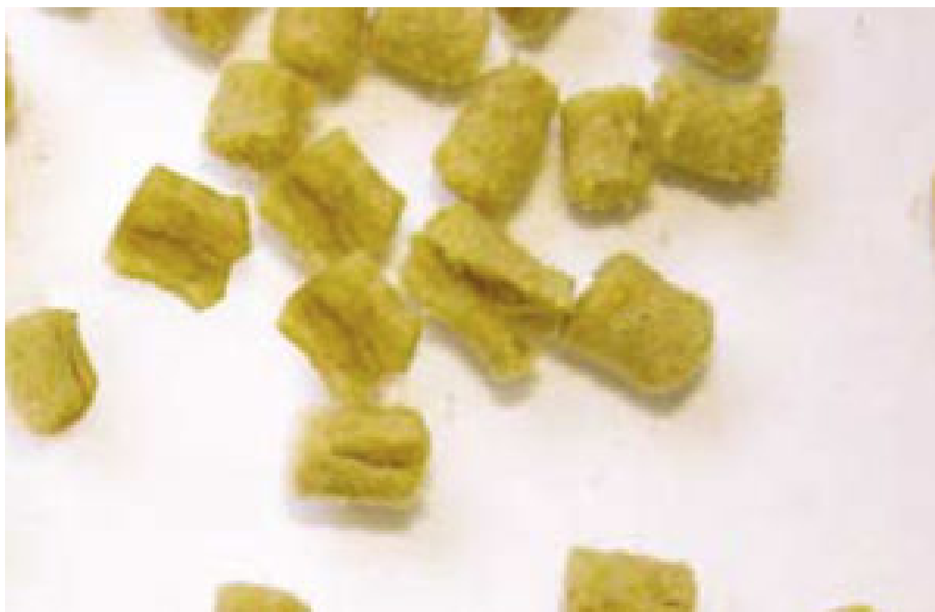
Fig. 2: Pellets produced under medium shear had longitudinal cracks after four hours of immersion.
