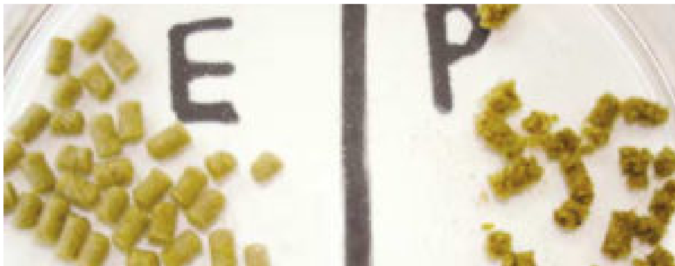
Fig. 3: Extruded pellets (E) produced under low energy input had better water stability than those pelleted using a pellet mill (P).
