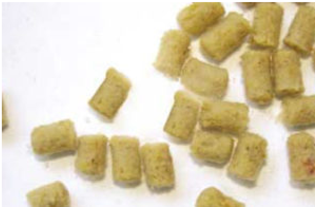
Fig. 1: Pellets produced under low shear held their physical integrity after water immersion.
