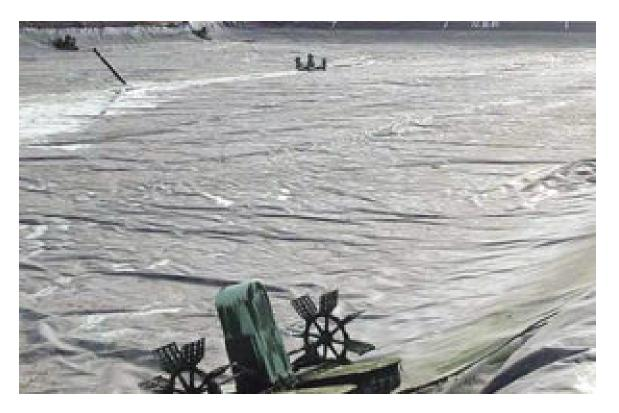
Many farms use earthen production ponds lined with high-density polyethylene plastic.
