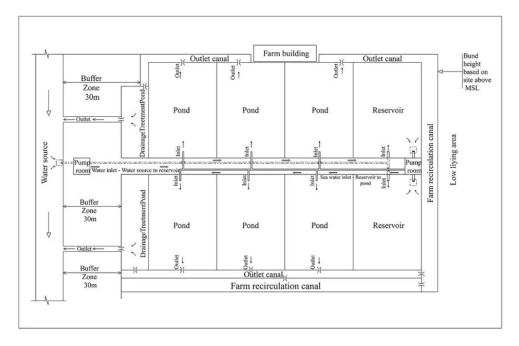
Fig. 1: Model design of small scale L vannamei farm with recirculation canal.
