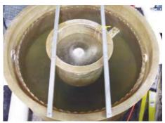
(Left) Fig. 1: As water rotates within a swirl separator, solids removal is mainly gravity-driven. (Right) Fig. 2: Radial-flow settlers are often used to settle microbiological solids during secondary water treatment.
