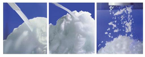
Variable-state ice slurry systems can generate product of varied consistency by controlling both the ice fraction and salinity of the discharged slurry.
