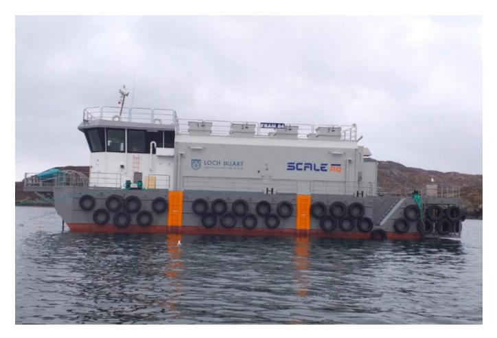
Loch Duart's new hybrid barge, which combines battery and diesel power, is estimated to cut the site's diesel consumption by up to 60 percent when compared to standard diesel systems. Photo courtesy of Loch Duart.
