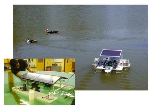
Solar panels on the "scarebot" charge batteries that drive paddlewheel controlled by electronic micro controllers guided by shore feeders or a GPS unit.
