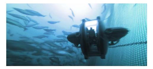
Deep Trekker manufactures portable underwater inspection tools like the DTX2 ROV – an underwater remotely operated vehicle (ROVs) that's battery-powered and widely used by aquaculture companies internationally.
