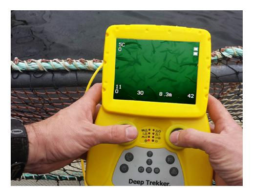
For fish farmers, ROVs have opened up "a whole new world." With anchors set at depths of up to 300 feet, drones can access and inspect areas that were previously inaccessible to divers, providing valuable information to their team. Live feeds can even be recorded for future viewing.
