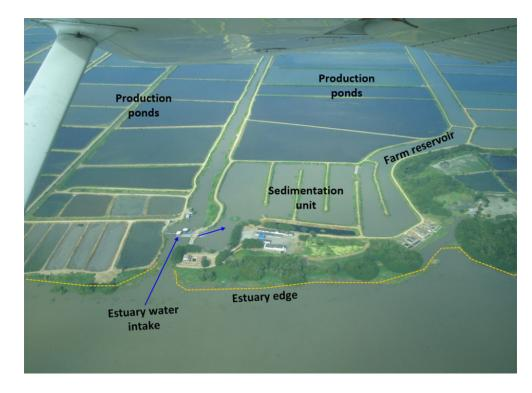
Aerial view of a retrofitted farm showing a sedimentation unit, production ponds and reservoir.
