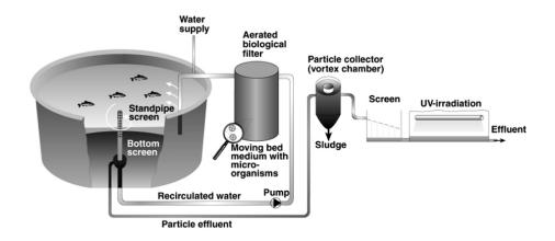
Fig. 1: The BIOFISH recirculation system.
