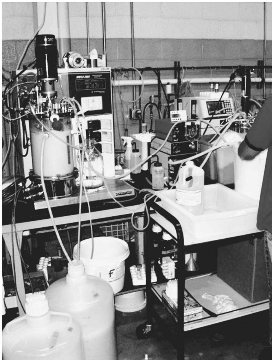
Separated soluble proteins and lipids are pumped to a second bioreactor for further pH adjustment to precipitate the muscle proteins.
