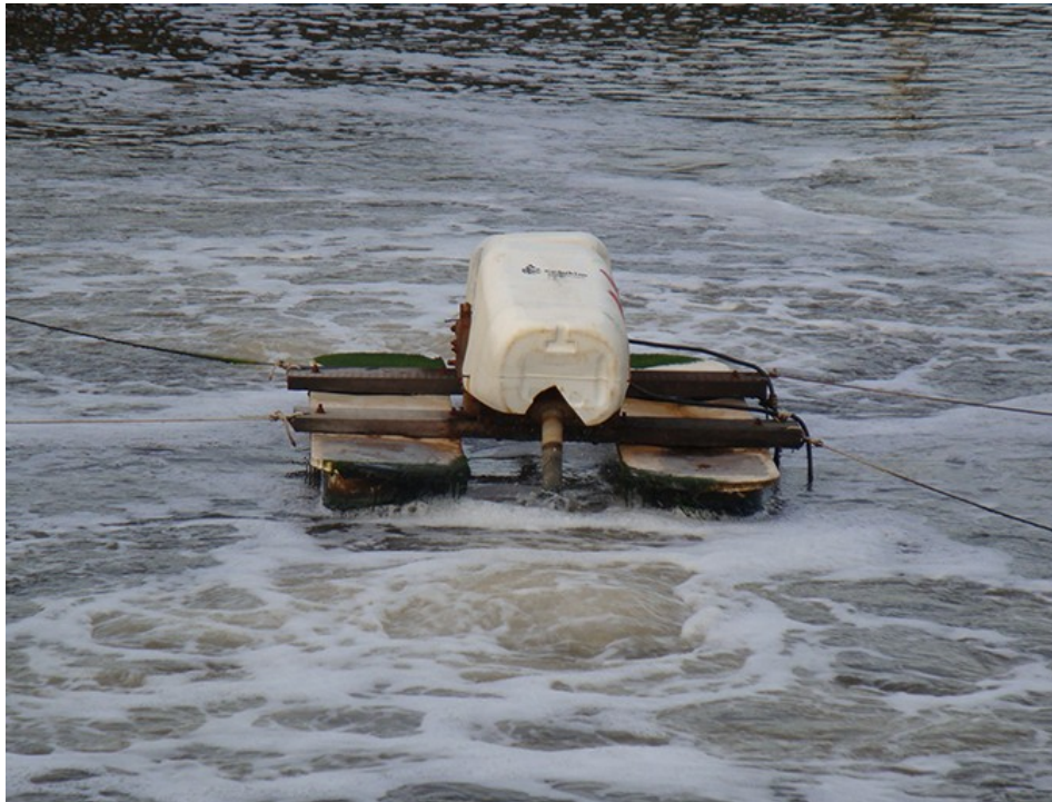
Fig. 7: Double-side mounted propeller-aspirators (2 hp each propeller) that is being used to promote the mixing of pond water. Propellers push surface water down without too much surface disturbance, causing minor losses of oxygen from DO-supersaturated surface water. Photos by Fernando Kubitza.
