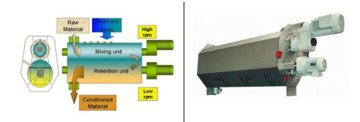
Many pre-conditioners have high radial mixing in a chamber where steam and water are injected. In a second chamber, more axial mixing occurs and the ingredient meal is hydrated there. Images courtesy of Buhler.
