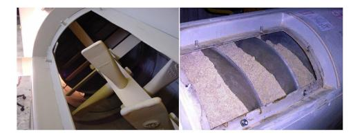
Views of the mixing (left) and retention zones (right) in a commercial pre-conditioner. Photos courtesy of California Pellet Mill.
