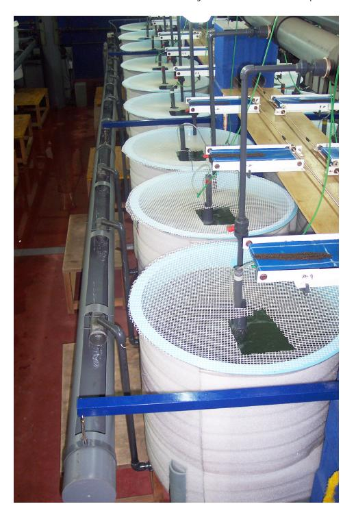
Automatic belt feeders provided each culture unit with a consistent source of feed for the test fish.
