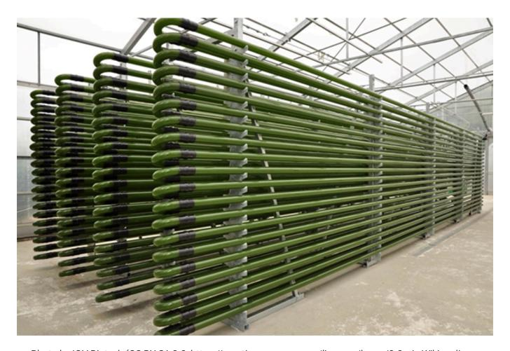
Photo by IGV Biotech (CC BY-SA 3.0, https://creativecommons.org/licenses/by-sa/3.0, via Wikimedia Commons) shows a tubular glass photobioreactor for the cultivation of microalgae and other photosynthetic organisms. This type of photobioreactor is suitable for the scaled production of microalgae-based high-value products.
