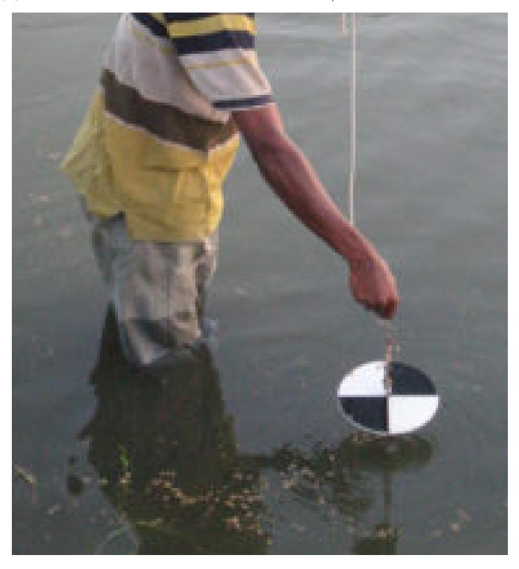
After initial fertilization establishes an adequate bloom, the frequency of fertilization can be adjusted based on bloom density and Secchi disk visibility.
