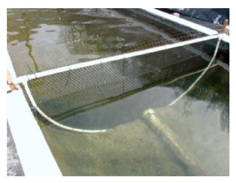
Hydrostatic water pressure pushed the solids that accumulated around the manifold into the off- solids removal pipe.
