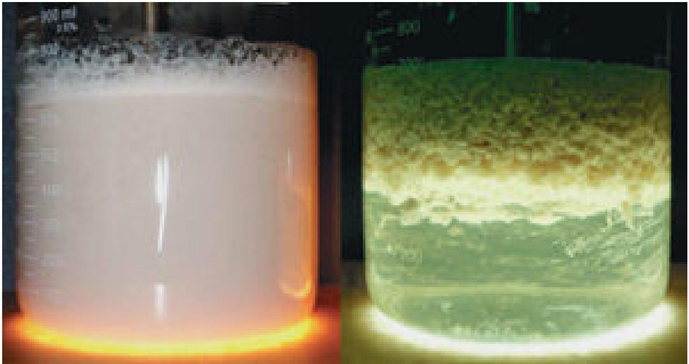
Protein flocculation can enhance separation of the fish muscle proteins in the decanter-centrifuge. On the left are fish muscle proteins without flocculant. On the right are muscle proteins following a 10-minute reaction with a commercial flocculant.
