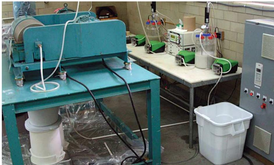
West Virginia University's recovery system shows a decanter-centrifuge on the left and two bioreactors on the right. The continuous homogenizer is not shown.
