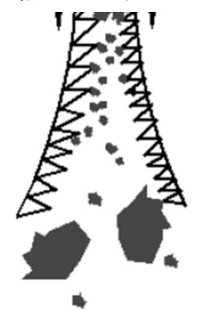
Fig. 2: Crumbler rollers rotate at different speeds and have different corrugations.
