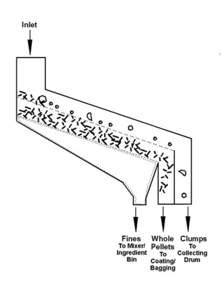
Fig. 3: Common screener separator.
