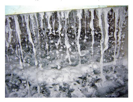
The discharge of a simple degasser helps partial pressures equalize by increasing air-water interface area.
