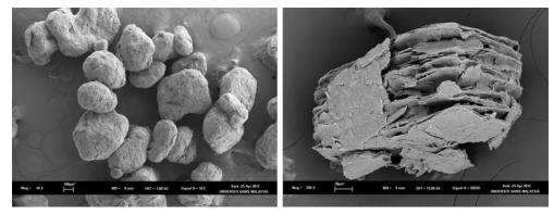
Scanning electron micrograph (SEM) of potassium diformate granules of a commercial organic acid salt product (Aquaform®, ADDCON) (Left photo) and a SEM showing the stacked, latticed, interconnecting pores of the special carrier used to adsorb organic acids used in the production of an organic acids blend (Biotronic<sup>™</sup>, BIOMIN) (Right photo). From Ng and Koh, 2017.
