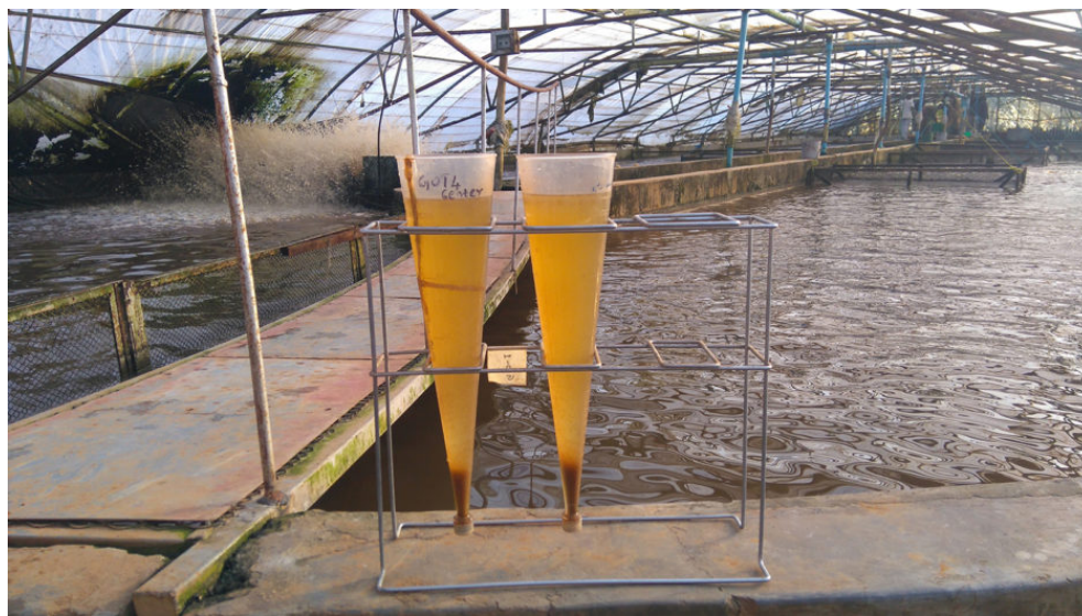
Fig. 4: Imhoff Cones used to measure floc volumes (mL/L) at Chambo Fisheries.
