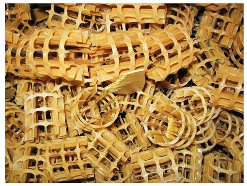
The high surface area of the water aeration media used to facilitate gas exchange in RAS systems also provides substrate for the growth of bacterial biofilms. Photo by The Conservation Fund.
