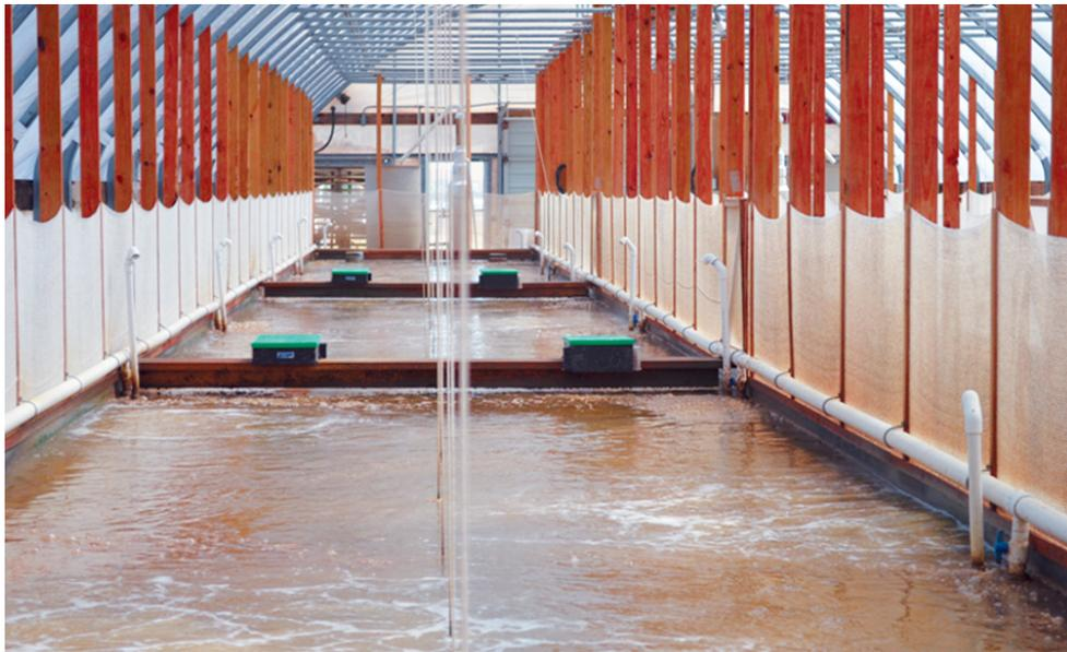
High-efficiency non-Venturi injectors are providing adequate aeration and water mixing in biofloc raceways.
