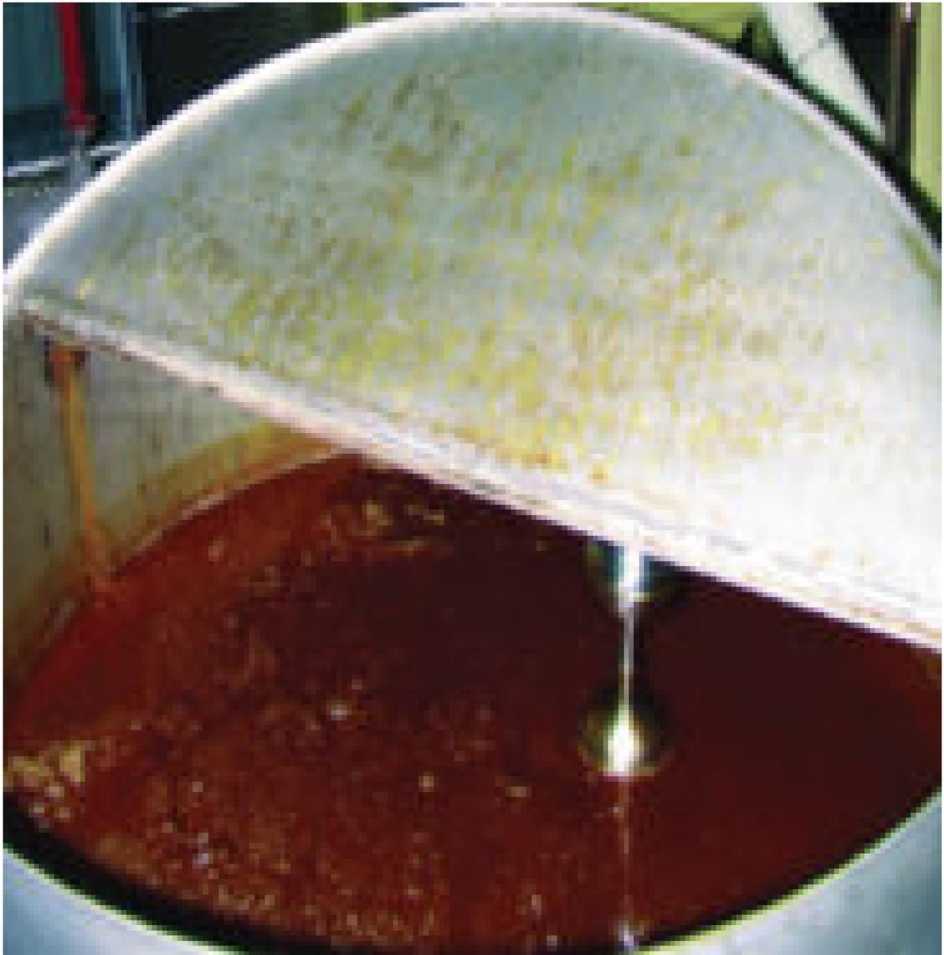
Fish oil like that in the foreground tank provides essential fatty acids. Feed pellets are fat-coated in the drum coater in the background.
