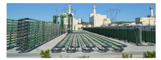
Photobiorreactors can be very efficient in removing nutrients and producing algal biomass. For example, 425 g N- NH4+/day and 125 g P-PO43/day can be removed in large-scale wastewater remediation with photoautotrophic *Scenedesmus obliquus*. Wastewater phytoremediation with species such as *Chlorella* sp. can achieve 80 percent NO3- removal with a biomass yield of 160 mg/L/day. Photo of commercial facility in Spain by AlgaEnergy, via Wikimedia Commons.
