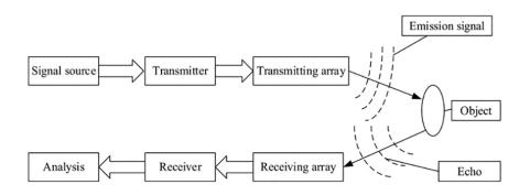
Fig. 1: Diagram showing how an echosounder works.
