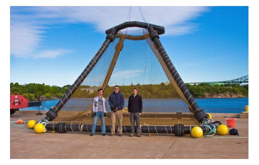
Copper alloy net cages offer increased strength and maintenance advantages, but may require special engineering for integration with existing facilities.
