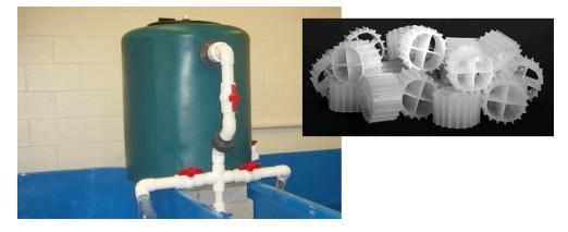
The plastic media in bioreactors is designed with high internal surface area to support microbial growth. The media mixes throughout the water column to treat waste loads efficiently without clogging.
