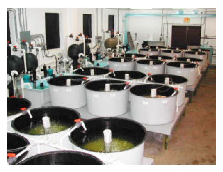
Larviculture production tanks at VSAREC are connected in threes to an intensive recirculating system that combines filtration and sterilization with individualized temperature and flow controls.
