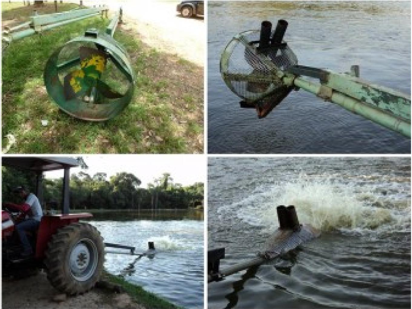
Tractor-powered, water circulator propellers such as this one can be used for either emergency aeration or for mixing pond water, just by regulating its operational depth. Circulators will force oxygen rich water to move down and contact oxygen depleted bottom water, increasing oxygen levels in pond bottoms. Photos by Fábio Mori.
