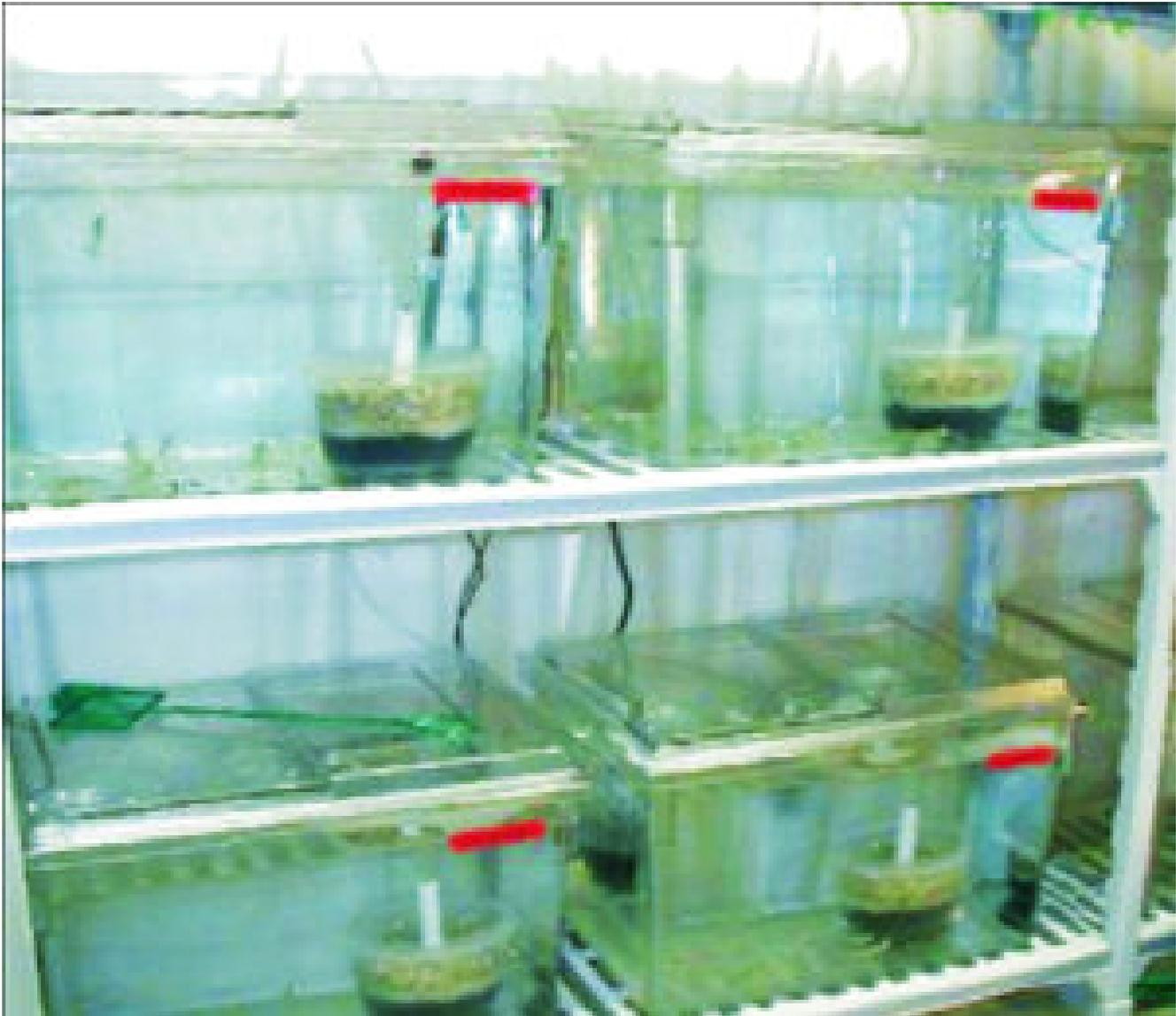
The experimental units consisted of covered 90-liter plastic tanks fitted with internal biological filters.
