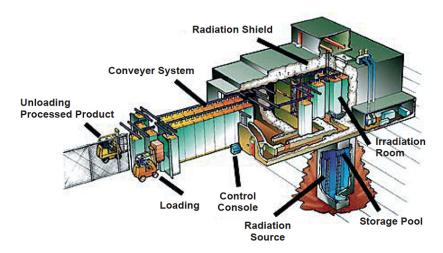
Typical gamma irradiation facility. Diagram courtesy of MDS Nordion, Ontario, Canada.
