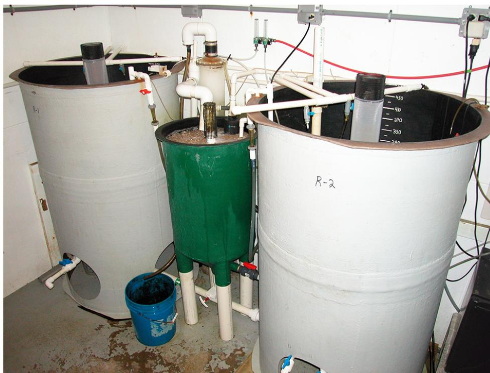
Rotifers are produced in an automated generator comprised of two 500-L culture tanks, a fluidized-bed biofilter and a protein skimmer.
